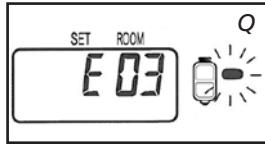
If the low fuel level indicator ⑯ lights up in combination with a short tone, then the fuel tank is empty. The heater will automatically burn at its lowest setting for a period of about 80 minutes. The fuel tank must be replenished.
